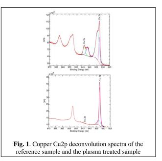
LMM triples at 916-920 eV, consistent with previous studies by Platzman et al. [2]. the oxygen concentration decreased from 35.8% for the reference sample to 21.1% after plasma treatment and one hour of air exposure confirming the reduction process.
